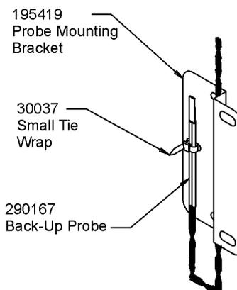
2. As shown in Figure 5-3, thread the small tie wrap through the openings in the front of the bracket. Secure the probe on the back of the bracket with the tie wrap. **Figure 5-3.** Secure probe
