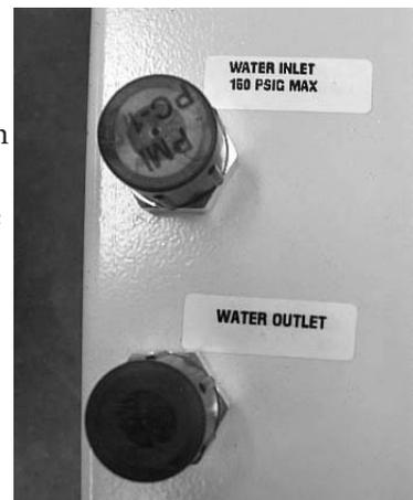
**Figure 5-2.** Inlet/Outlet Fittings
