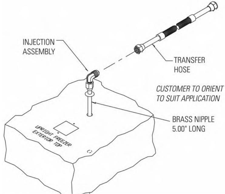
Figure 5-1. Injection Assembly
